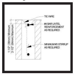
**STEP 3:** Install upper lintel rebar.
